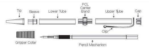
**Pencil Assembly** *Note: Line up parts according to layout above.*
