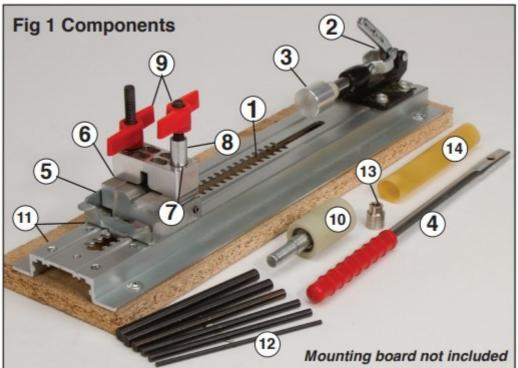
It is recommended that the press be mounted or clamped to a work space to prevent slipping and aid in leverage. Slide a 2"x18" piece of thin wood or cardboard under the platform to capture parts that fall into the slot.
