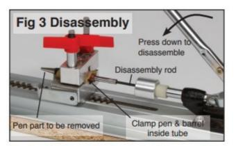
Fig 4a-4b 7mm Mechanism disassembly
