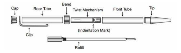
A. Press the tip into the front tube.
